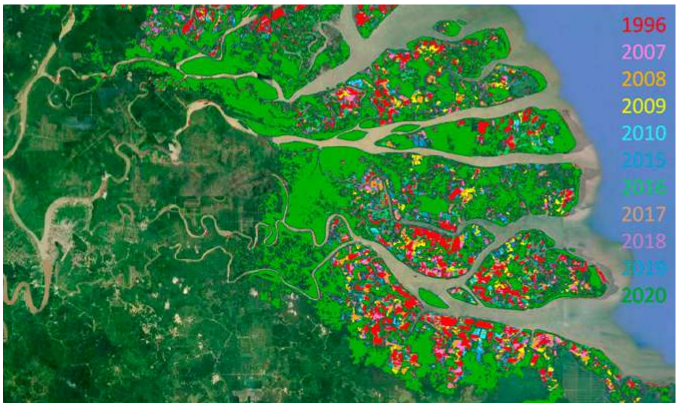
Global Mangrove Watch, mapping the extent of mangroves from 1996 to present using observation data by JERS-1, ALOS and ALOS-2, with the advantage of being able to obtain data on the ground surface regardless of weather conditions
